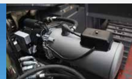
Electric pre-heating system Engine start below -50°C temperature Engine coolant hiting system by diesel fuel Webasto installed
