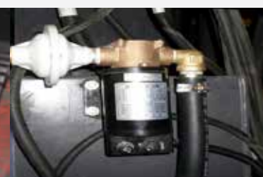
Electric re-fueling pump Fuel pump operated by electric control (For refilling fuel in a job site)
