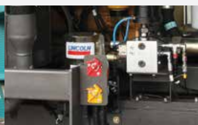
Start motor shut down switch To cut electric line completely for parts safety during maintenance
