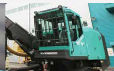
Safety guard Protecting cabin glass from relatively bigger flying object
