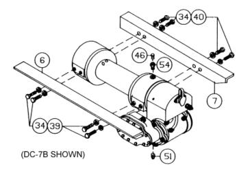
Attach mounting angles (items #6 & #7) using eight capscrews (item #34) with lockwashers (item #39 & #40). Torque capscrews to 12 ft. lbs. (16 Nm.) each. Insert plug (item #51) into bottom of gear housing. Permatex may be applied to threads to help prevent leakage.
