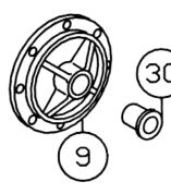
11.Check cover bushing (item #30)for signs of wear. Replace if necessary by removing old bushing and pressing new bushing into place.
