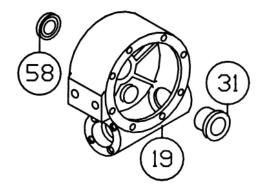
8. Remove seal (item #58) from back of gear housing (item#19). Press bushing (item #31) from gear housing. Press new bushing and seal back into place.
