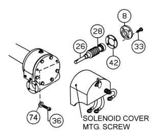
16. Press bearing (item #28) onto worm (item #26). NOTE: Be sure thick shoulder of bearings outer race (side with manufacturer's name and part number) is out, away from worm threads. Press bearing and worm into gear housing. Slip gasket (item #42) onto bearing cap (item #8). Use four capscrews (item #33) to secure cap to gear housing. Torque capscrews to 8ft. lbs. (10.8 Nm.) each.
