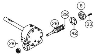
Remove bearing cap (item #8) and gasket (item #42) from gear housing by unscrewing four capscrews (item #33). Remove worm (item #26) and bearing (item #28) from gear housing. Use a soft hammer to gently tap input end of worm and drive worm and bearing from gear housing. Once worm has been removed from housing, bearing can be pressed from end of worm.
