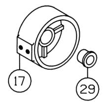
Check end bearing bushing (item #29) for signs of wear. If necessary, remove old bushing and press new bushing into place.
