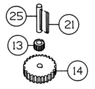
13. Check gears (items #13 & #14) of spur gear shaft assembly for signs of wear, replace if necessary. Press old gears from shaft (item #25). Tap key (item #21) into keyway of shaft (item #25). Press shaft through gears so that gears are centered on shaft and key.
