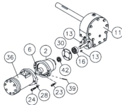
4. See page 12 for servicing the oil cooled brake. Remove brake housing mounting screws (item #22) and remove brake with gasket. Replace gasket (item #30). Remove worm (item #15) and bearings (item #16) from gear housing. Use soft hammer to gently tap input end of worm and drive worm and bearing from gear housing. Once worm has been removed from housing, bearing can be pressed from end of worm.
