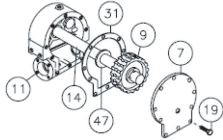
6. Check for signs of wear on gear teeth. If replacement of gear is necessary, replace as follows:
