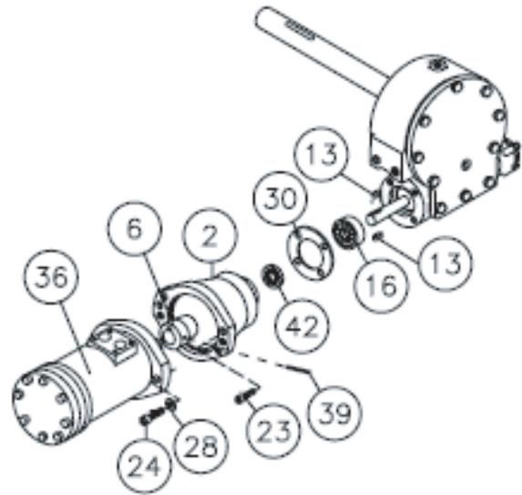
Insert keys (item #13) into keyways of worm shaft. Slide tapered end of coupling (item #6) over end of worm shaft. Be sure roll pin (item #39) is in coupling.
