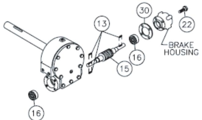
13. Press bearing (item #16) onto worm and into housing. NOTE: Be sure that thick shoulder of bearings outer race (side with manufacturer's name and part number) is out, away from worm threads. Place gasket (item #30) onto adapter (item #2). Attach adapter to gear housing using four (4) capscrews (item #23). TIGHTEN CAPSCREWS TO 12 FT. LBS. (16.3 Nm.) EACH.
