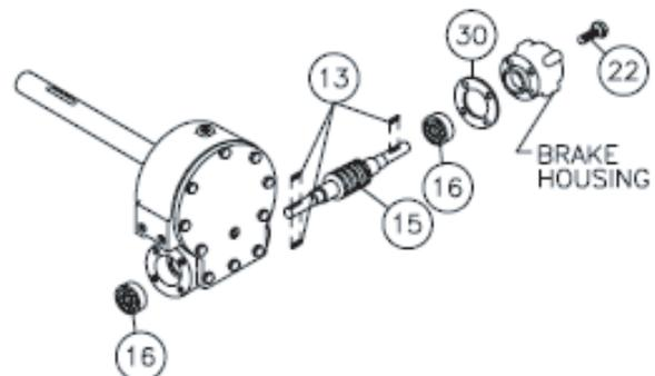
Check for signs of wear or damage to worm (item #15) and bearing (item #16). Replace if necessary.
