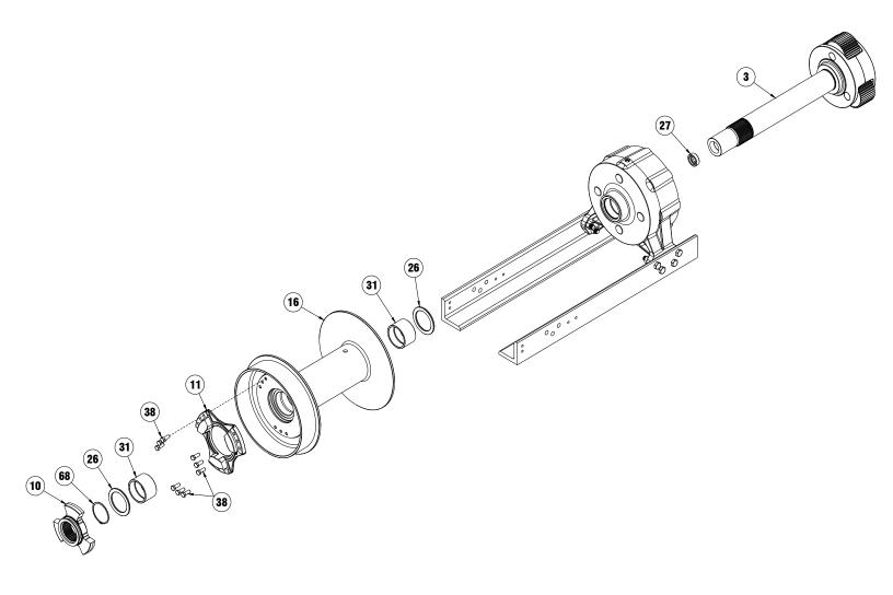
To remove gear end bearing #21, from mounting angles #7 and #8, first remove (4) bolts #40 and (4) nuts #42 from each angle. Shaft oil seal #66 and end bearing bushing # 31 can be removed and replaced at this time, if necessary.
