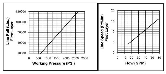
**BASED ON 7.0 CU IN/REV MOTOR**
