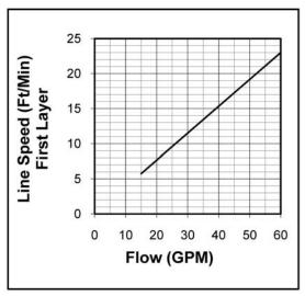
**BASED ON 9.0 CU IN/REV MOTOR**
