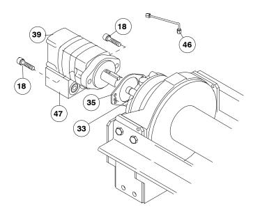
Remove brake assembly screws from brake #33 to access (2) mounting screws #17 attaching brake to end bearing #8. Caution: Brake is spring loaded by clutch spring and must be restrained against end bearing as mounting screws are removed. Remove coupling #6 and gasket #35 from end bearing. Take note of mounting configuration for proper mounting of parts during reassembly.
