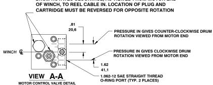
WITH PLUG AND CARTRIDGE IN POSITION SHOWN CABLE DRUM ROTATES CLOCKWISE, AS VIEWED FROM MOTOR END OF WINCH, TO REEL CABLE IN. LOCATION OF PLUG AND CARTRIDGE MUST BE REVERSED FOR OPPOSITE BOTATION
