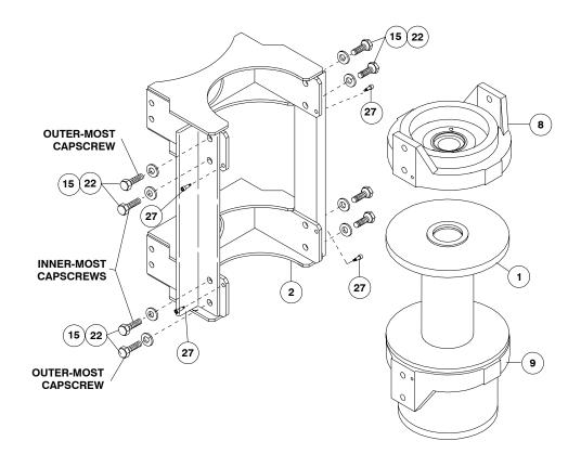
5. Pull drum assembly #2 upward from end bearing #9. Remove quad-rings #40 from grooves in drum bushings. Remove input shaft #10, clutch springs #44 & #45 and washers #25 & #26 from end bearing. Examine splined ends of input shaft for signs of wear, replace if damaged.
