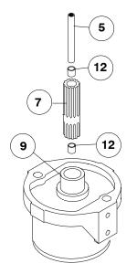
7. Remove (12) capscrews #14 to pull gear-housing cover and gasket from ring gear. Remove input thrust washer, sun gear and carrier assemblies from inside of ring gear. Remove ring gear #3 and gasket #34 from end bearing #9. Examine shifter shaft #11 for signs of wear, replace if necessary. Examine bushing #13 for signs of wear. Replace bushing, if necessary, by pressing old bushing from housing and pressing new bushing into place.
