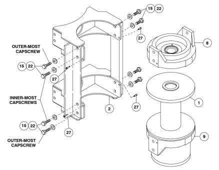
9. Place end (with longest splines) of output coupling assembly #7 through end bearing bushing #13 and mesh coupling spline with spline inside of drum. Slide clutch spacer #28 over end and against shoulder of shifter shaft #11. Place shifter shaft through washer #25 and into shaft coupling #5, meshing splines of shifter shaft with splines in shaft coupling.
