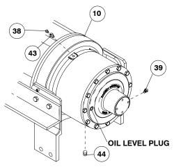
relief fitting #38 are not damaged and in good operating condition. Replace if necessary.
