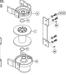
Place end (with longest splines) of output coupling assembly #6 through end bearing bushing #13 and mesh coupling spline with spline inside of drum. Slide clutch spacer #29 over end and against shoulder of shifter shaft #12. Place shifter shaft through washer #24 and into shaft coupling #6, meshing splines of shifter shaft with splines in shaft coupling.
