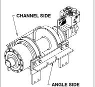
R. H. MOUNTINGL. H. MOUNTINGCONFIGURATIONCONFIGURATIONWINCH MOUNTING CONFIGURATIONS
