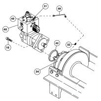
Remove brake mounting screws #19 from brake #34 to remove brake from end bearing #9. Take note of mounting configuration for proper mounting of parts during reassembly.
