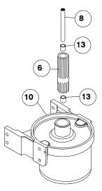
Remove (12) capscrews #17 to pull gear housing cover and gasket from ring gear. Remove input thrust washer, sun gear and carrier assemblies from inside of ring gear. Remove ring gear #4 and gasket #35 from end bearing #10. Examine shifter shaft #12 for signs of wear, replace if necessary. Examine bushing #14 for signs of wear. Replace bushing, if necessary, by pressing old bushing from housing and pressing new bushing into place.
