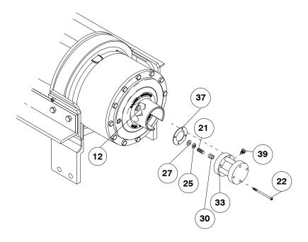
12. Liberally apply grease to shoulder of input shaft. Place 1-3/4 OD washer #26 over end of shaft and against shoulder of shaft. Place spring #46 inside of spring #47 and place both springs over shaft and against washer #26. Slide 2-3/8" OD clutch washer #24 over splined end of shaft and against springs. Use grease to hold springs and washers in place on shaft. Place end of shaft through drum. Mesh spline of input shaft with internal spline of coupling shaft inside of drum.
