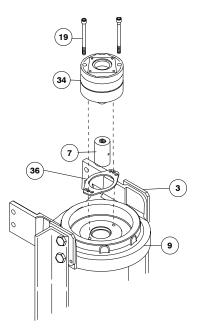
Remove winch from tie bars #2 and #3 by removing (8) capscrews #18, (8) lockwashers #23, and (4) shoulder bolts #28. Pull motor end bearing #9 from drum assembly #1.
