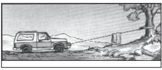
For basic self recovery, anchor to a tree or heavy rock. When anchoring to a tree, always use a tree trunk protector.
