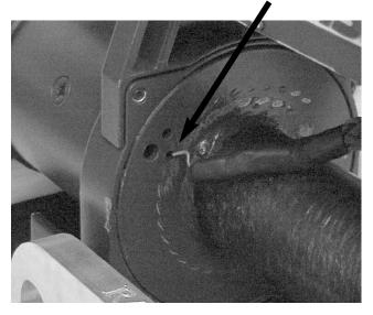
Pull synthetic rope tight to seat anchor in hole.
