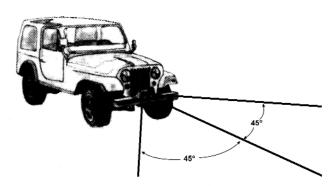
Winches equipped with fairleads can pull from several directions. Pull from an angle only to straighten up the vehicle-otherwise you can damage structural members or other parts of your vehicle and cause excess rope buildup on one end of the winch drum.
