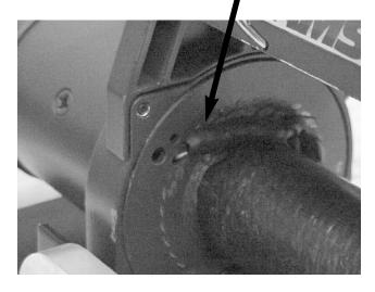
6. Carefully run winch in the "reel-in" direction. Wear gloves and use the hook strap, keep tension on end of rope as you spool all the rope onto the drum, taking care to form neatly wrapped layers.
