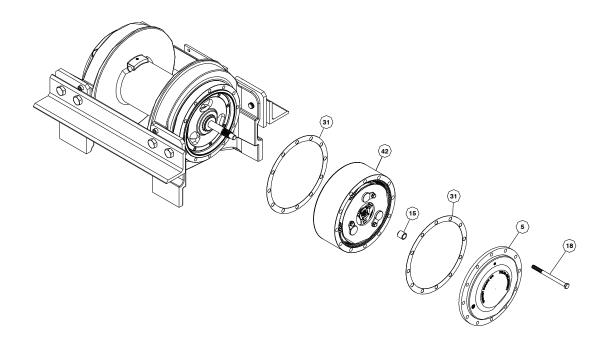
4. Remove (8) capscrews #20 to remove clutch retainer plate #10 from clutch piston. Remove clutch #9.
