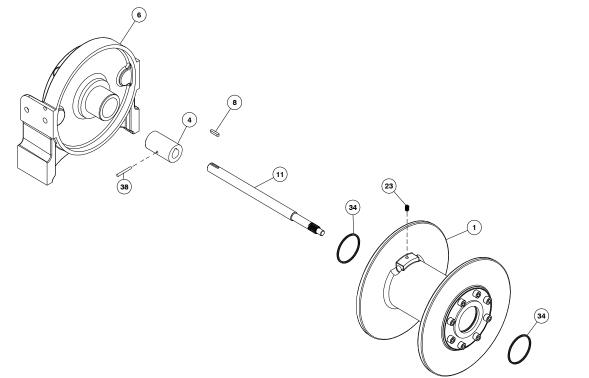
9. If splines inside drum driver #102 are damaged, drum driver must be replaced. Remove drum driver by unscrewing (8) capscrews #105. If bushings show signs of wear, replace by pressing old bushings from drum #101 and removing o-rings from grooves in drum and drum driver. Place well oiled o-rings #106 into driver and drum. Place well oiled o-ring #107 on outside of driver. Press bushings #104 into drum driver until flange is flush and #103 is flush against drum.
