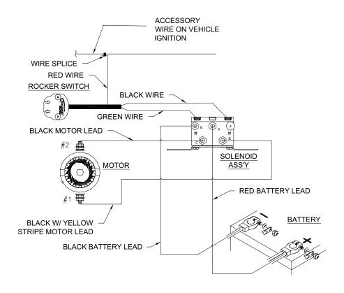
**For certain mounting applications,** where the solenoid needs to be mounted at the rear of the vehicle, switch the battery and motor leads. In this case, connect the black w/yellow stripe lead to the positive (+) terminal of the battery, and the longer black lead to the negative (-) terminal. Connect the red lead and the shorter black lead to the motor terminals.
