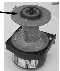
3. Remove the bolts that hold the end plate to the motor end housing. Lift off the end plate and take the nuts and washers out of the mounting feet. Set aside the gear assemblies and bushing. The input sun and planetary gear carrier may come out together.
