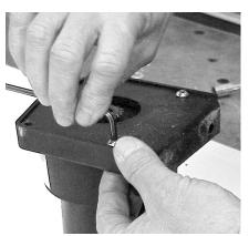
4. Lean the motor end and loosen the motor tie bolts off the tie bolt nuts. Lean the motor end back up so that it is sitting upright. Do not let the motor end cap come apart from the rest of the motor. Lift the motor end housing and rotate 90°. Put the tie bolt nuts in the other set of pockets and carefully lean the motor end back. Tighten the tie bolts to 45-50 in-lbs. torque. Do not overtighten.
