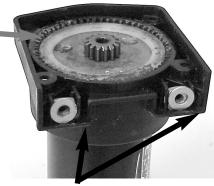
Insert the mounting nuts and washers into the pockets of the housing as shown. Make sure they do not fall out while re-installing the end plate.
