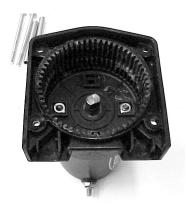
After rotating the motor, the motor end will appear as shown at right. The motor studs will be aligned horizontally, and the motor tie bolt nuts will be in the other set of pockets.
