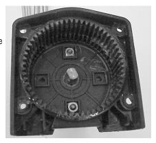
Replace the gears into the motor end housing, fitting the input sun gear over the motor shaft. The planetary gear carrier should be seated so that the bushing, as shown at lower right, is flush with the ring gear.
